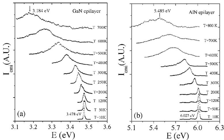
FIG. 1. (a) PL spectra of GaN epilayer measured from 10 to 700 K. (b) PL spectra of AlN epilayer measured from 10 to 800 K.
