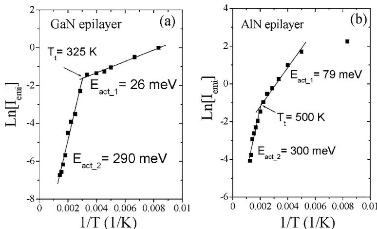
FIG. 2. (a) Arrhenius plot of the integrated PL emission intensity ( $I_{emi}$ ) of the dominant band edge transition in (a) GaN and (b) AlN. The solid lines are the least squares fit of the data with Eq. (1) for two different temperature ranges. Measured values of activation energies ( $E_{act,1}$  and  $E_{act,2}$ ) are also indicated.
