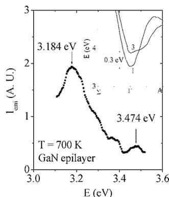
FIG. 3. PL spectrum of GaN epilayer at 700 K. A new emission peak at 3.474, which is 0.29 eV above the dominant band edge transition at 3.184 eV, is evident. The inset shows the conduction band of GaN near the  $\Gamma$  point (after Ref. 14).
